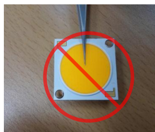
Fig.5 Improper Handling of the COB Using Tweezers
