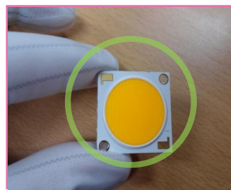
Fig.4 Proper Handling of the COB Using Anti-Static Gloves
