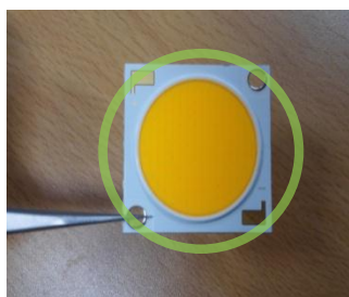
Fig.3 Proper Handling of the COB Using Tweezers
